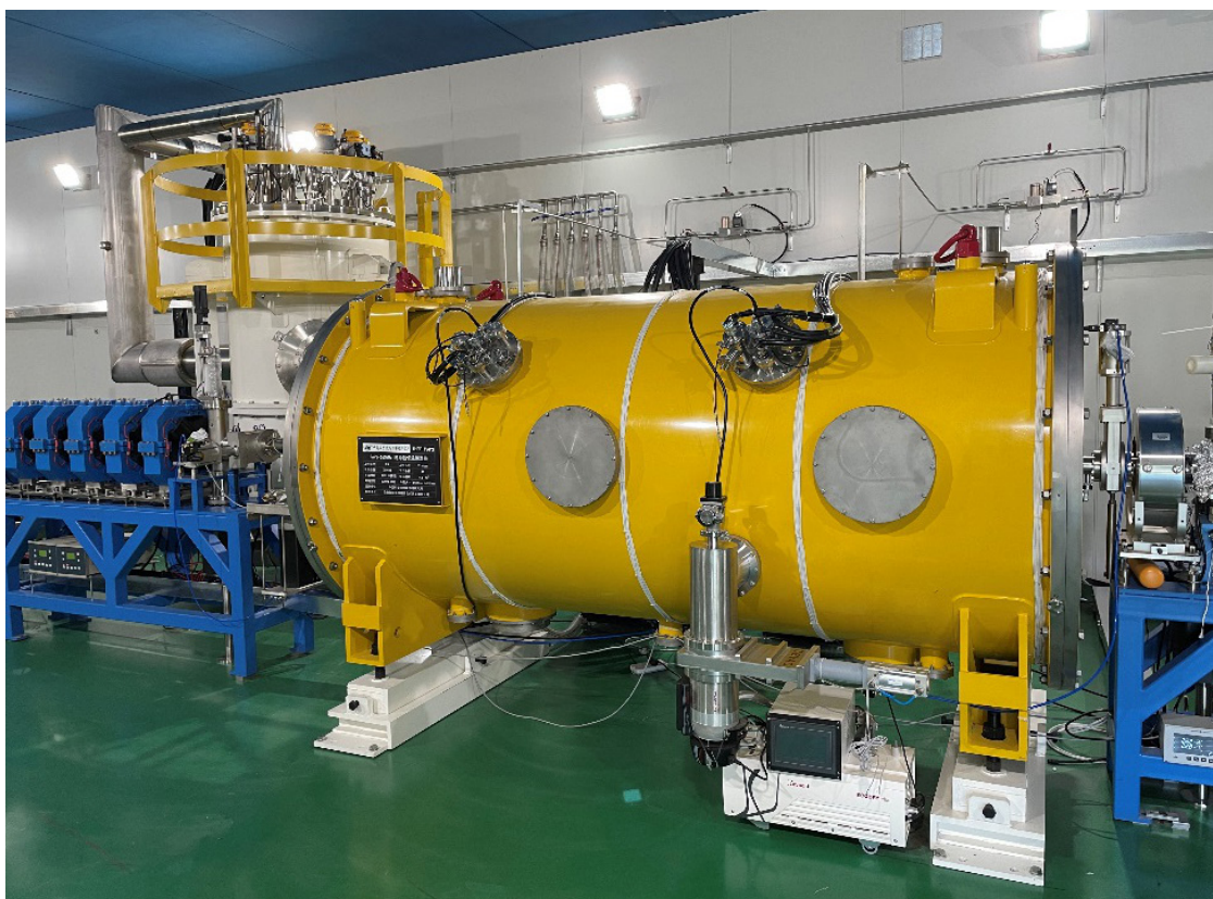
650 MHz 超导腔模组样机（包含 2 个 650 MHz 2-cell 超导腔及附属设备） Prototype of 650 MHz cryomodule, which consist of two 650 MHz 2-cell Superconducting cavities and accessories.
